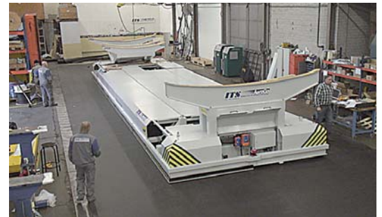
AeroGo delivered an AGV, with a length of 16 meter, on air bags supporting and moving airplane structures, up to 40 tons, between different work stations.
