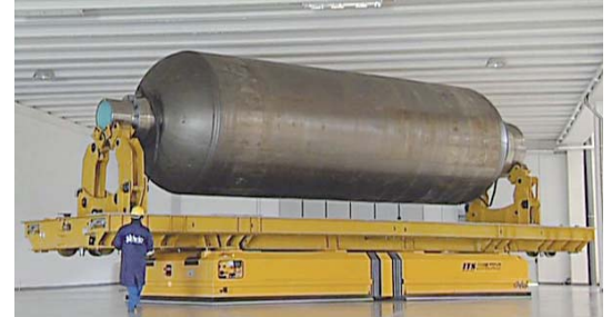
A 130 ton "Aero-Pallet" transporter of AeroGo moves moulds of fuel tanks for the Ariane rocket between the different work stations. The transporter is extensible from 8.4 up to 12 meter.
