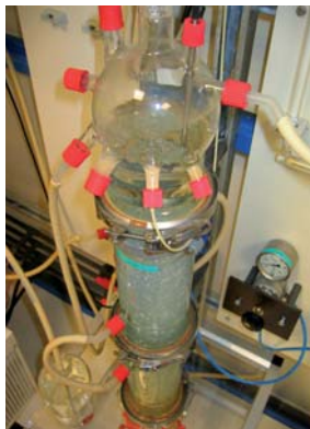
Bioreactor with micro-organisms for the treatment of waste water
