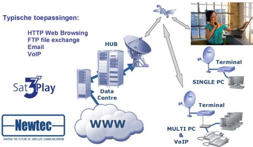
mounted on a 75cm antenna. The iLNB is the integration of a standard LNB and a low-power, small-size 0,5 Watt transmitter. Indoors, a small-size Sat3Play DVB-S2 Indoor Unit connects to the end-user's PC via a standard Ethernet port and to the outdoor satellite antenna via standard coaxial cables.
